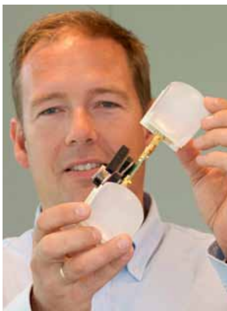
The development kit includes a Radar RF-module with a Novelda Radar IC, Antennas, an IO module for communication with a PC.
