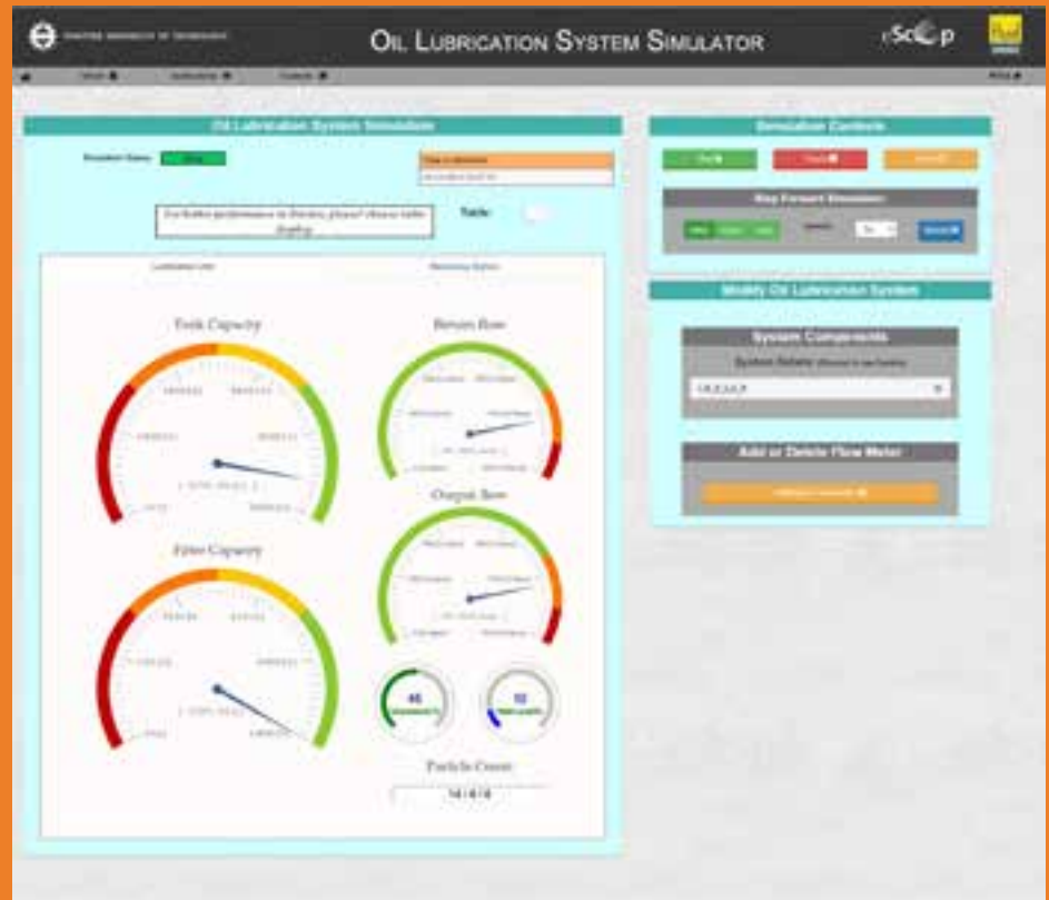
Figure 1: Graphical User Interface of the Oil Lubrication Simulator visualises the parameters of simulated system, configured by the user.
