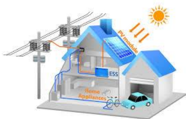
Figure 24 - The Prosumer concept. The Power transmission goes from one-way to two-way lines
