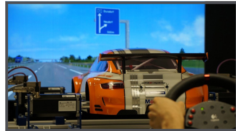
Figure 1 – Mini DrivingCube sample setup with VTD
