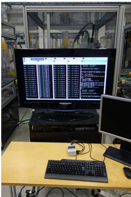
Figure 3. Raspberry PI (small grey box between keyboard and the screen) hosts the orchestrator and testers for the FASTory line. It is probably the cheapest item seen in the photo.
